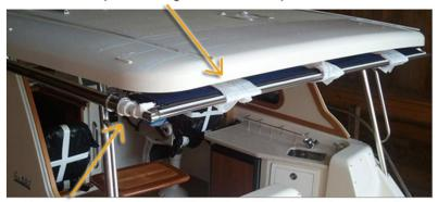
Use preservation tape to close off gaps around the actuators to prevent water penetration between the extending tubes, especially when the boat is rigged aft-facing toward the front of the truck. Highway transportation in this manner and during inclement weather can result in excessive amounts of water to enter the actuator and compromise the actuators' internal components.
