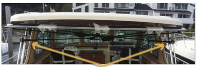
Stabilize the SureShade framework from vibration during ground transport by securing a strap on one side of the framework and tying the strap off to the opposite side of the boat. Repeat this so both sides are tied off and crisscross in the middle as shown above.
